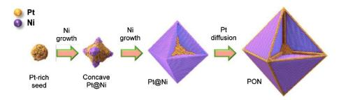
**Figure 3.** Schematic diagram illustrating the formation of a Ni-rich phase-segregated octahedral nanoparticle (PON), showing the formation of a Pt-rich frame with <110> edges and <100> inner axes. Reprinted with permission from Ref. [62]. Copyright 2015 American Chemical Society.
