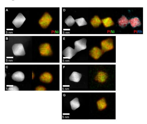
**Figure 5.** HAADF STEM images and EDX maps of (A–C) Pt–Ni and (D–G) Rh-doped Pt–Ni nanoparticles. (A, D) show the initial state, while (B, E) were acquired after 4 k, (C, F) after 8 k and (G) after 30 k cycles. Although the Pt–Ni nanoparticles become spherical after 4 k cycles, the Rh-doped Pt–Ni nanoparticles retain their octahedral shapes even after 30 k cycles. Reprinted with permission from Ref. [78]. Copyright 2016 American Chemical Society.
